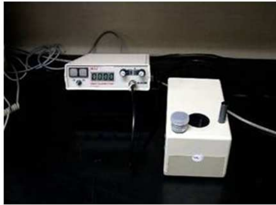
Figure 2: Bartington Susceptibility Meter
